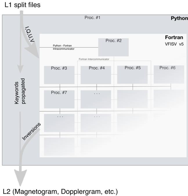
**Figure 1:** Workflow showing the pipeline running on  $N$  processors, with the main python processor spawning the VFISV inversion on  $N - 1$  processors.
