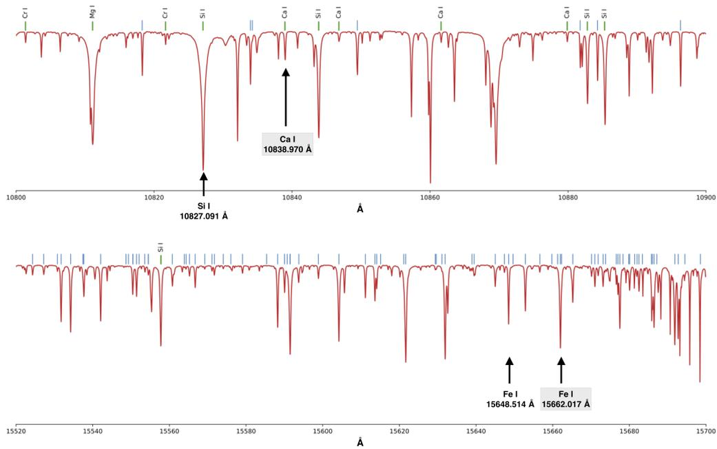
**Figure 2:** The two spectral ranges covered by GRIS showing the prominent lines. The standard inversion product delivered by SDC are for the Ca I 10838.970 Å line for the 10830 Å range and the Fe I 15662.017 Å line in the 15650 Å range.
