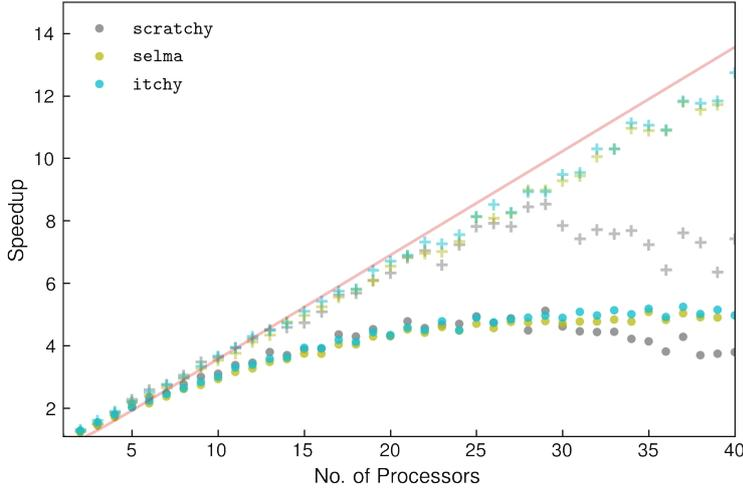
**Figure 6:** Speedup as a function of processors on three different machines. The dots represent the full pipeline performance, including the I/O. The plus markers represent only the inversion part of the pipeline.
